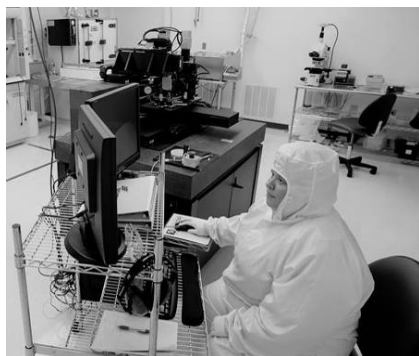
FIGURE 3. Micro-transfer print tool developed at Semprius.
